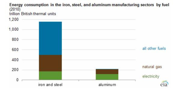
The energy demand required for producing aluminum is far more efficient than iron & steel production.
